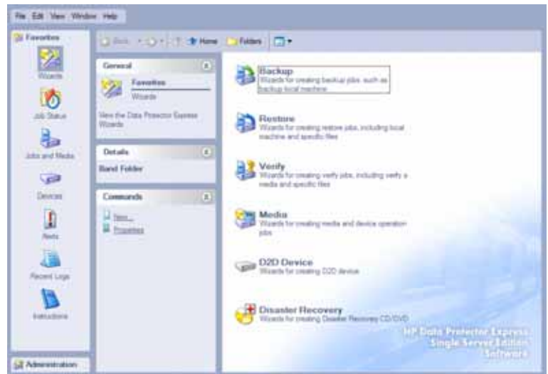
Figure 2a. Wizards are available, from the Favorites desk bar, to automate the most frequently run tasks.
